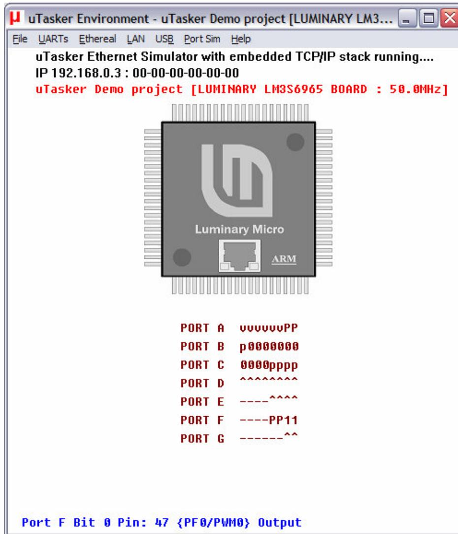
If you hover your mouse over the port which is toggling, or other available ones, you will see which pin number it has on the device, its name and present use, as well as the possible peripheral functions which it can be programmed to perform. In the screen shot above this is seen by the line in blue at the bottom of the simulation window.
