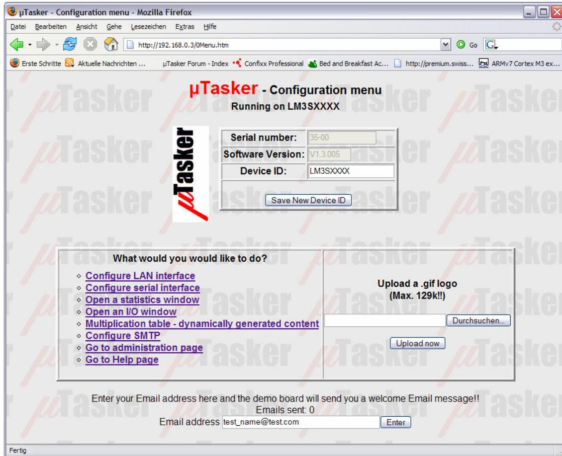
**Serial number** – this is a decimal representation of the MAC address programmed in the device. Since the MAC address is normally unique it can serve also as a serial number if required. Notice that the serial number is displayed in grey and can not be modified (disabled).
