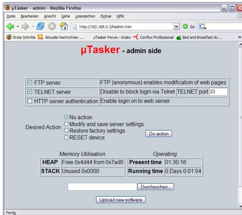
It is possible to upload new software as long as the project is compiled with the boot loader support. See the boot loader documentation for details of how to activate and use this.
