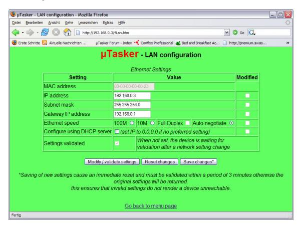
This side is a very critical side since it allows important Ethernet settings to be modified. The first time the device is started, the default MAC address – defined in the cParameters structure in **application.c** - is 0-0-0-0-0. It can be changed just once, after which it is displayed as disabled. This is because it is normally necessary to program a new device with a unique MAC address which should normally never be changed again.
