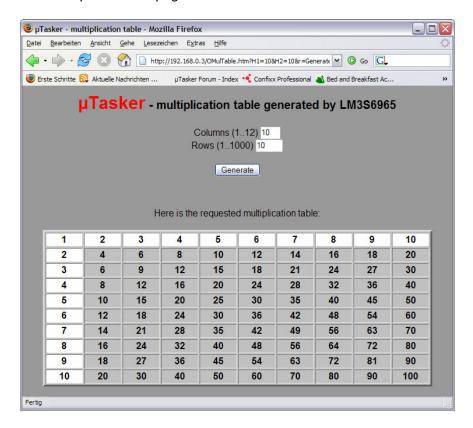
The values for Columns and Rows have been used to generate a multiplication table with these dimensions. The demonstration accepts column values from 1 to 12 and row values from 1 to 1000 and shows how user code can quite easily interface to the HTTP server and generate its own HTML (or Java script etc.) content.
