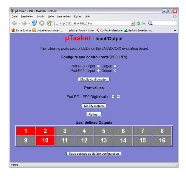
Set PF1 to be an output, rather than an input and click on "Modify configuration". Afterwards set the port state to '1' by un-checking the third port value from the right and click on "Modify outputs".
