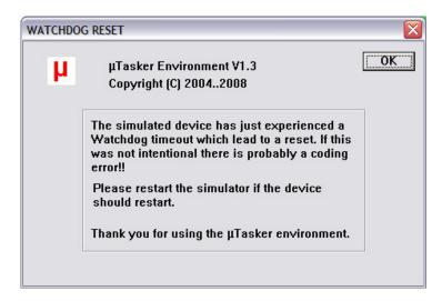
You can restart the simulator after the reset (which was interpreted as a normal program exit and so the changes to the FLASH have also be saved to the hard disk and will be restored on the next program start) by using F5 as normal.
