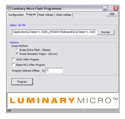
Step 4: Press the program button and wait until the programming has completed. This is seen in the bottom status line.
