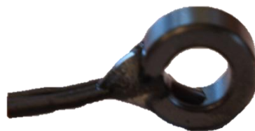
Abbildung 5: Hall-Sensor in Ferritring
