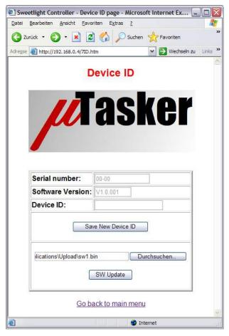
A standard Web Browser input allows the user to select a file to be loaded from the user's hard disc. In this example the user has already selected a file with the name sw1.bin - the format of which has been prepared to include the necessary header.
