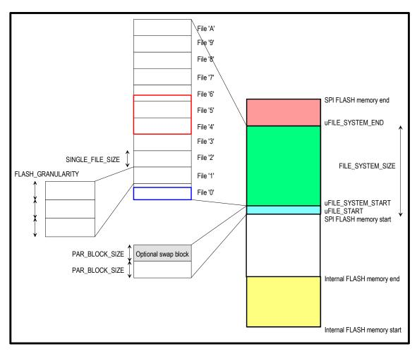
Location of µFileSystem in external SPI FLASH – example 1
