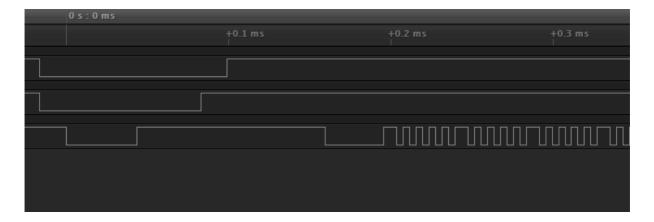
Thi shows a break set/clear generates 43us (10 bits), which is the only possibility in LPUART (43, 86, 129us etc would be possible by queuing multiple – but timing critical...)
