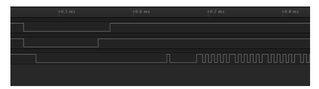
Using PIT to control delays and the LPUART's break generation.
