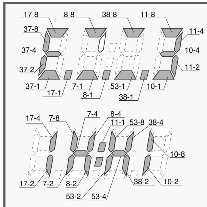
Example: Segment control 8-8 is the bit 0x08 (phase controlled by COM 3) in the register LCD\_WF8, which corresponds to the 67th control bit in the control block. To enable it the following can be used: `SET_SLCD(8, 0x08)`, to clear it `CLEAR_SLCD(8, 0x08)` and to toggle it `TOGGLE_SLCD(8, 0x08)`.
