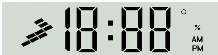
This example shows 3 x 7-segment digits. The first '1' is a single segment, as are the ':', '°', '%', "AM", "PM" and freescale logo. This means that there are 28 individual segments, which are controlled by particular bits in the SLCD controller's registers `LCD_WF15TO12` and `LCD_WF23TO20`.
