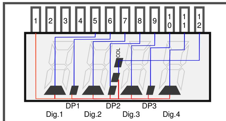
This means that when the COM0 line is being driven up to 8 segments can be turned on, depending on the state of the 8 segment pins. The 8 segment pins (5..12) thus control these 8 segments during this driving phase and can turn all on, all off, or an combination in between.
