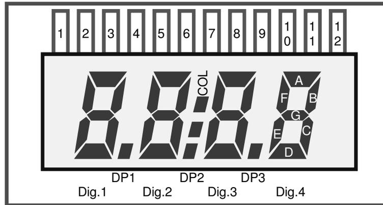
This display has 12 pins, which are all connected to a driving pin on the SLCD controller. There are 4 common pins and so the driving mode is  $\frac{1}{4}$  duty, since each of the common pins are driven for  $\frac{1}{4}$  of the cycle period. Each of the common lines is connected to 8 LCD segments. Taking COM0 as an example the 8 segments that are controlled by it are show in the following diagram.
