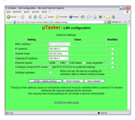
This side is a very critical side since it allows important Ethernet settings to be modified. The first time the device is started, the default MAC address – defined in the cParameters structure in **application.c** - is 0-0-0-0-0. It can be changed just once, after which it is displayed as disabled. This is because it is normally necessary to program a new device with a unique MAC address which should normally never be changed again.
