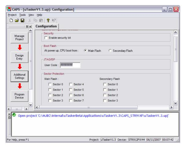
Here it is visible that the chip is to be configured to boot from the main FLASH. This is the default configuration of the chip so is already valid if the chip has not previously been programmed with a different configuration.
