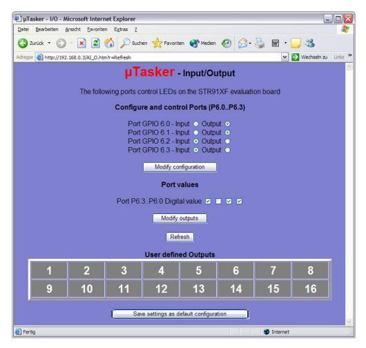
Set GPIO 6.2 to be an output, rather than an input and click on "Modify configuration". Afterwards set the port state to '1' by setting the third port value from the right and click on "Modify outputs".
