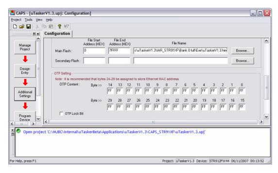
Step 6. Finally click on the "Apply" button which causes the CAPs too to create a file of its own which will later be downloaded to the target. This step is more interesting when using code in both the main and in the secondary FLASH since this step causes these two parts to be merged into one downloadable file.
