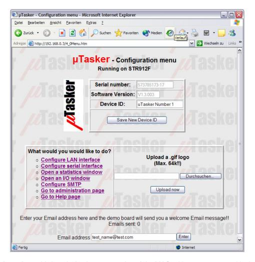
**Serial number** – this is a decimal representation of the MAC address programmed in the device. Since the MAC address is normally unique it can serve also as a serial number if required. Notice that the serial number is displayed in grey and can not be modified (disabled).
