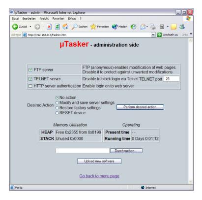
It is possible to upload new software as long as the project is compiled with the boot loader support. See the boot loader documentation for details of how to activate and use this.
