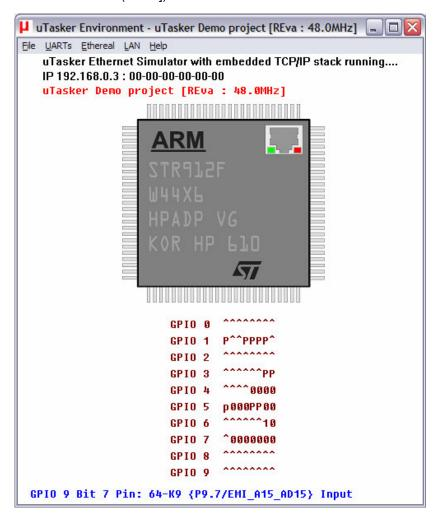
If you hover your mouse over the port which is toggling, or other available ones, you will see which pin number it has on the device, its name and present use as well as the possible peripheral functions which it can be programmed to perform. In the screen shove above this is seen by the line in blue at the bottom of the simulation window.
