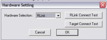
Ensure that the RLink is selected (If you happen to have a FlashLINK this is also supported). You can use the two testes "RLink Connect Test" to ensure that your PC is correctly connected to the RLink and "Target Connection Test" to verify that the CPU is also powered and responding.
