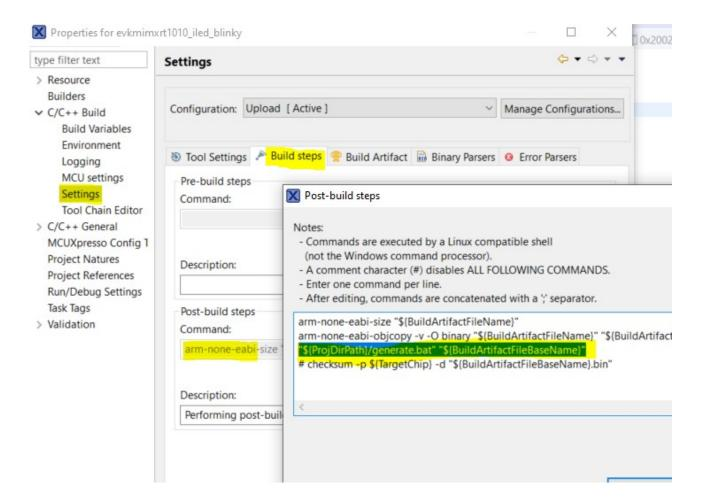
3. In the Post-build steps option the binary output is enabled and a bat. file call added:
