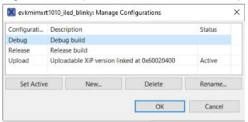
The first modification is to adjust the memory map so that the code is linked to run from the uTasker loader's application address, which is usually  $0 \times 60020400$  ( $0 \times 70020400$  for i.MX RT 1064 running in internal QSPI flash). This is performed in the target properties C/C++ Build  $\rightarrow$  MC Settings:
