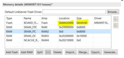
Note that the offset of 0x400 ensures both library and interrupt vector compatibility, when the vectors are in QSPI flash. A value fo 0x200 is also possible with the i.MX RT 1011 since it has less vectors, but generally a fixed layout is used to avoid any potential confusion.
