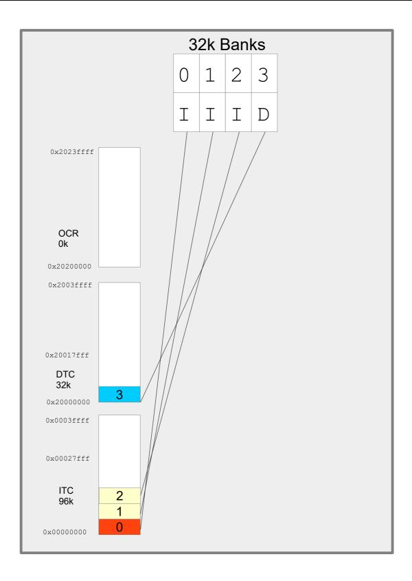
The  $\mu$ Tasker FlexRAM driver always uses the bank order from instruction use to data use (if OCRAM were used it would be inserted between the two). The most important thing to understand is that when the bank use is modified the address range of the bank is also changed (it is moved in the memory map). This means that data that was in OCR before the change (in the default configuration) still exists in the bank memory but is now addressed in the ITC or DTC memory space instead.
