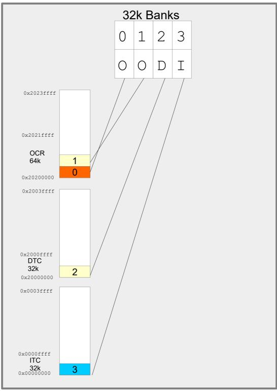
This default setting is assumed in the µTasker project to avoid special configuration requirements and therefore out of reset the banks are configured to give this memory map and layout:
