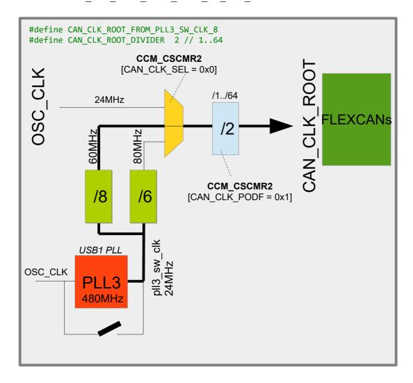
In this configuration the USB1 PLL is used as reference (called <code>pll\_sw\_clk</code>) and divided by a fixed value of 8, resulting in 60MHz. An optional pre-scaler defined by CAN\_CLK\_ROOT\_DIVIDER can divide this by 1 to 64 (when not defined, the default is 2)
