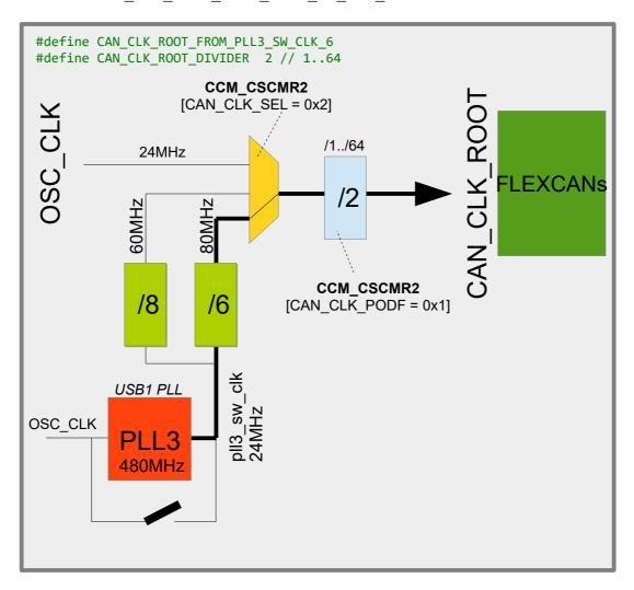
In this configuration the USB1 PLL is used as reference (called  $pll_sw_clk$ ) and divided by a fixed value of 6, resulting in 80MHz. An optional pre-scaler defined by CAN CLK ROOT DIVIDER can divide this by 1 to 64 (when not defined, the default is 2)
