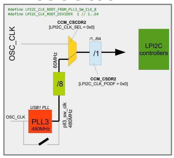
In this configuration the USB1 PLL is used as reference (called  $pll_sw_clk$ ) and divided by a fixed value of 8, resulting in 60MHz. An optional pre-scaler defined by LPI2C\_CLK\_ROOT\_DIVIDER can divide this by 1 to 64 (when not defined, the default is 1)
