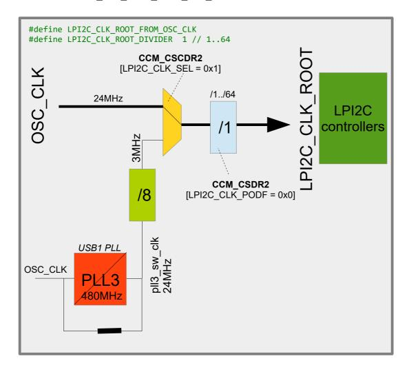
In this configuration the OSC\_CLK (24MHz) is used as reference, with the optional pre-scaler of 1 to 64.
