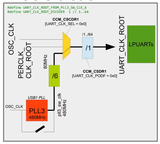
In this configuration the USB1 PLL is used as reference (called  $pll_sw_clk$ ) and divided by a fixed value of 6, resulting in 80MHz. An optional pre-scaler defined by UART\_CLK\_ROOT\_DIVIDER can divide this by 1 to 64 (when not defined, the default is 1)
