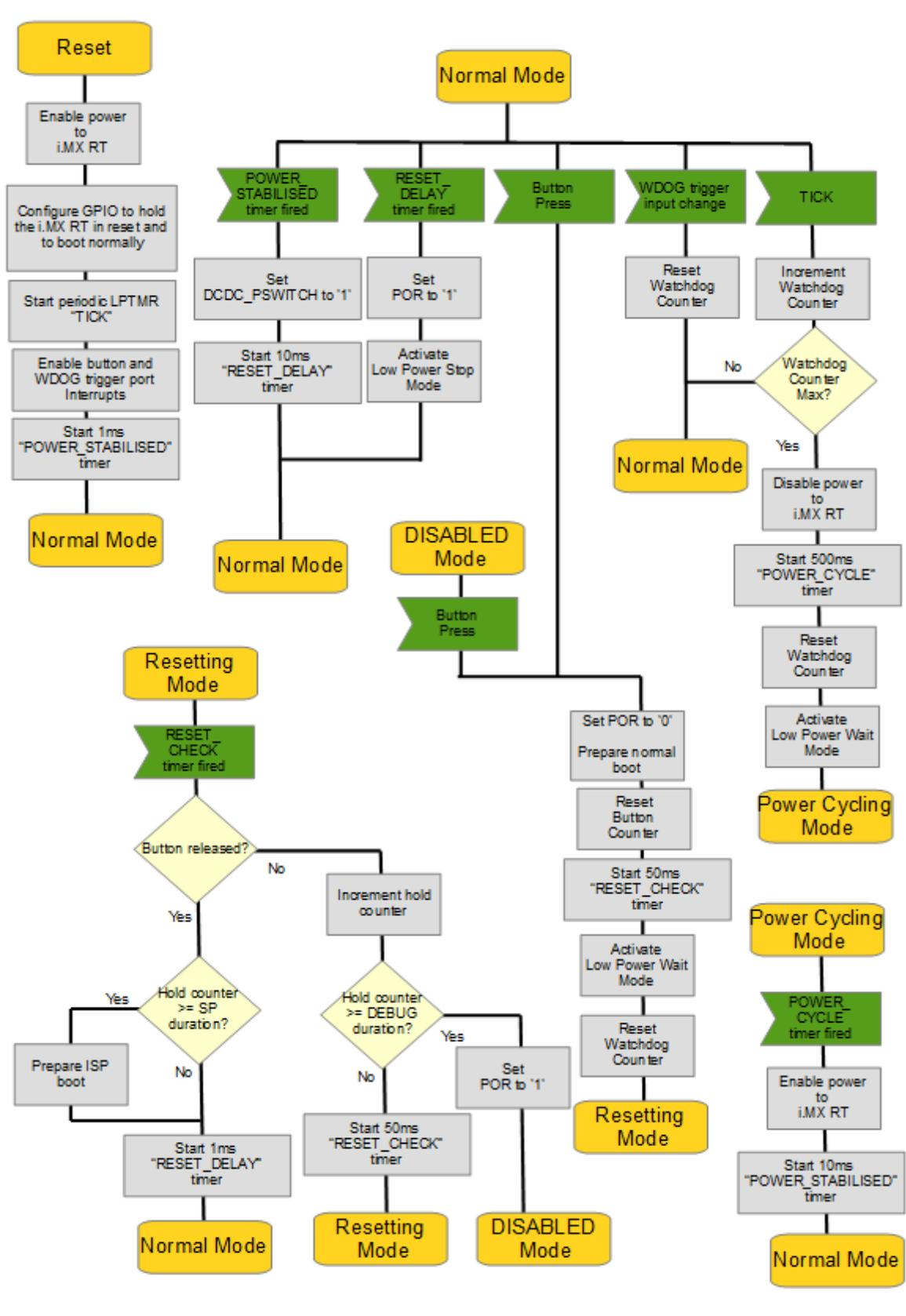
Typically the push button is used to perform a normal reset (guaranteeing > 50ms reset pulse) when pressed momentarily and held less than 3s.
