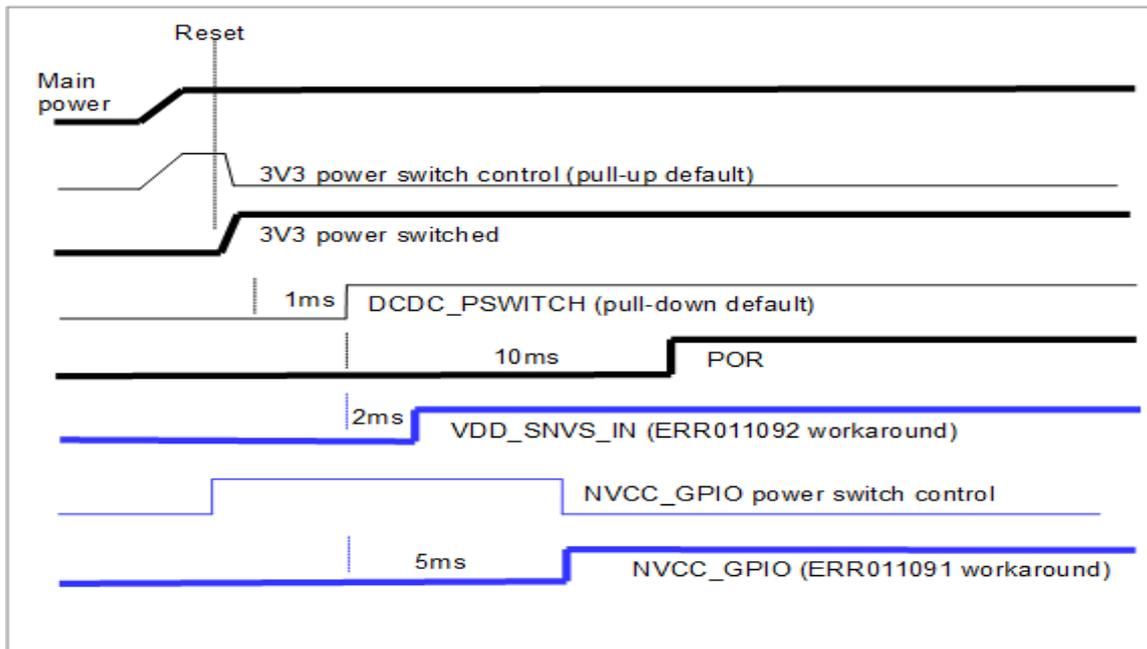
As soon as the controller starts it enables the main power to be switched to the i.MX RT but doesn't enable the DCDC in the i.MX RT via the `DCDC_PSWITCH` input *until after a delay of 1ms* to allow it to first stabilise. During this time the i.MX RT is held in its reset state via the `POR` input and for a further 10ms to allow the DCDC output to become ready.
