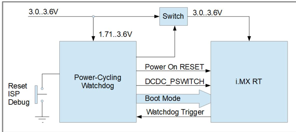
The circuitry consists of the power-cycling watchdog, which is a Kinetis KL02Z8VFG4 or KL03Z8VFG4 (in miniature 3.0 x 3.0 x 0.65mm 16-pin QFN package) performing specific power cycling/sequencing steps, monitoring the correct operation of the i.MX RT and controlling its reset and boot mode according to user input from a *single* push button switch.
