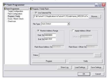
When programming, the target "uTasker\_BM.elf" should be programmed, rather than "uTasker\_full.elf". To be sure that neither attempts are made to program to the boot loader sector or to the file system area, the address range has been restricted (example for internal FLASH – Start 0x1000 is correct for SPI FLASH), although not absolutely necessary if the correct file is selected.
