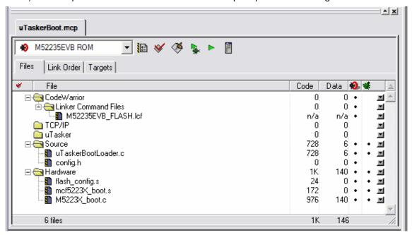
Once this project has been compiled, it can be loaded to the target using the normal loading sequence (see the  $\mu$ Tasker tutorial for the M5223X) and then occupies the first 2k of FLASH (4k with external SPI FLASH support).
