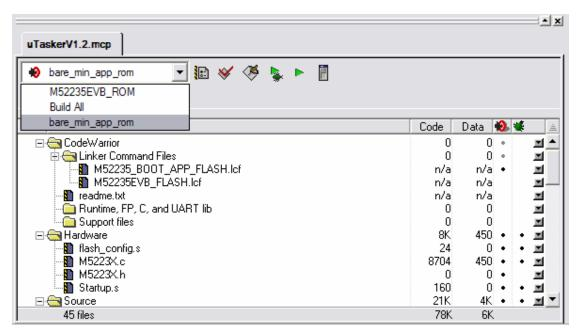
This project window shows the  $\mu$ Tasker demo project which has two target configurations: M52235EVB and bare\_min\_app\_rom.
