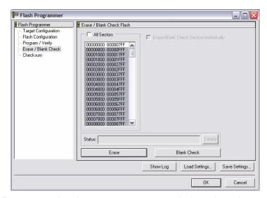
Here the Flash Programmer has been set up to erase only the selected sectors. The first sector containing the boot loader is not selected and so will not be deleted (the first 2 sectors should not be selected when using SPI FLASH).
