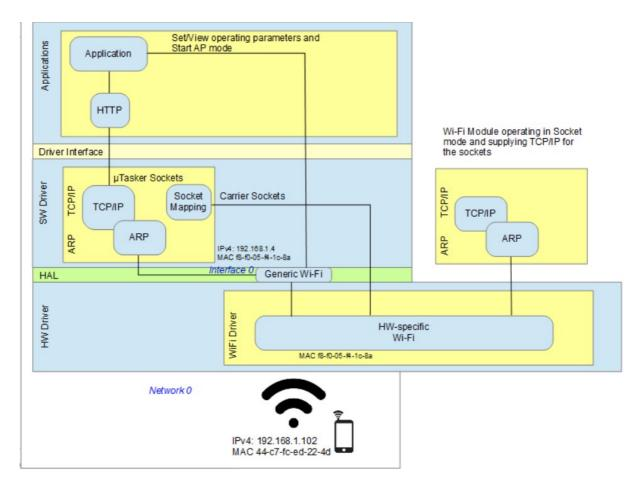
This diagram illustrates the situation when a Wi-Fi module is operating in socket mode and handling one or more TCP sockets for use by HTTP and an application (eg. a web server).
