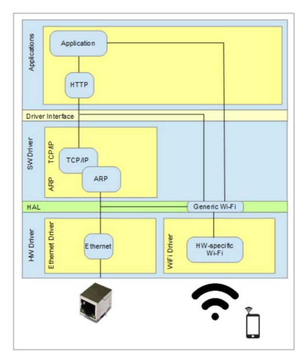
The Generic Wi-Fi interface sits between the HW-specific driver and the TCP/IP stack so that raw frames can be routed in a similar fashion to an Ethernet interface.
