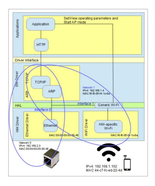
8.3 Processor with an Ethernet and a Wi-Fi Interface allowing Mobile Devices to Communicate with LAN Devices and use the LAN router of Internet Access
