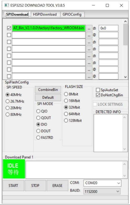
Make sure that the COM port matches that on which the connected ESP32-S2 module enumerates as ("Silicon Labs CP210x USB to UART Bridge) and start the loading process by clicking on "START".
